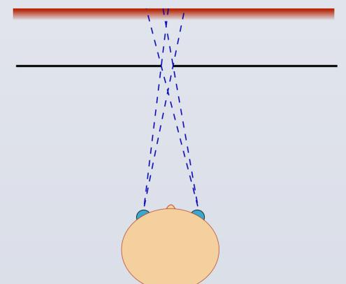
Figure 6. Visible parts of the screen through opened vertical slit in the shutter
