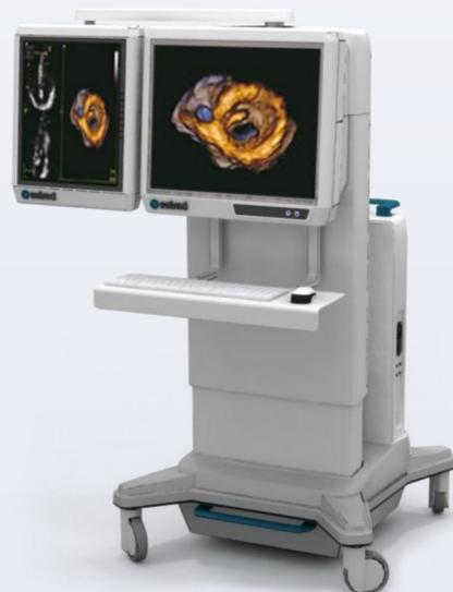
Figure 4. 3D ultrasound data being presented on holographic 3D display
